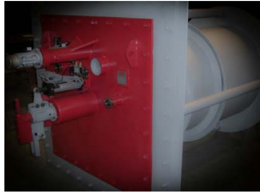
Figure 1 - STEP Low NOx Burner
